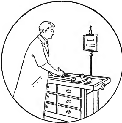
BLUE-PRINT HOLDER ATTACHED TO PATTERN-MAKER'S OR WOOD-WORKER'S BENCH, HOLDING MOUNTED BLUE PRINT.
